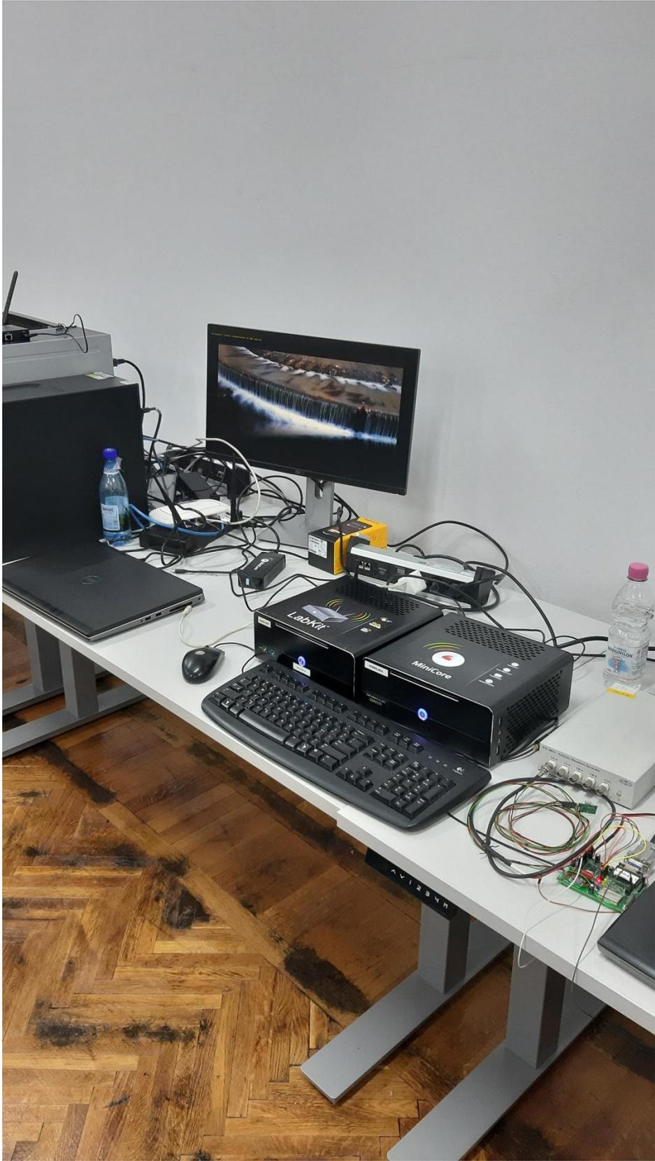
Figure 5: The 2 main equipments for the laboratory LTE network: the eNB (center left) and the core network (center right). Also, on the right side, the demo platform for biometric data collection (the chest pulse measuring belt not visible)
